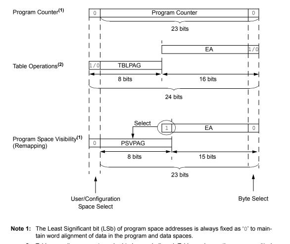
**2:** Table operations are not required to be word aligned. Table read operations are permitted in the configuration memory space.
