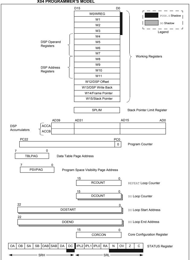
FIGURE 2-2: dsPIC33FJ32MC302/304, dsPIC33FJ64MCX02/X04, AND dsPIC33FJ128MCX02/ X04 PROGRAMMER'S MODEL
